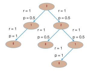
Note that in an MRP tree, the same state can appear multiple times, but each copy of the same state is identical — that is, the subtree rooted at each copy must be identical. In Figure 14.2, the state 1 appears twice in the tree. Every time it appears, it can only lead to state 0 with probability 1. This is simply the result of fixing a policy  $\pi$  — once we know the state we are in, we only have one choice for the action to take.
